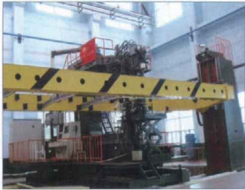
图1 企业改造的钻铆机及托架系统 Fig.1 Automatic riveting machine and bracket system after enterprise reform
